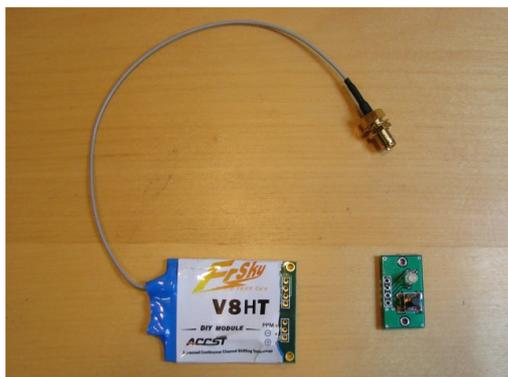
If you're doing the same on the PPM connector, note that the Frsky order doesnt match standard servo cable. On the module it goes pos, neg, signal (ppm) as can be seen from the label. Servo cable goes neg, pos, signal - so you have to cross-over the pos & neg:
