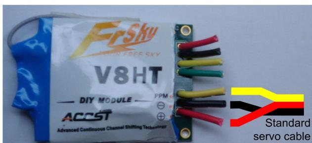
Remember that by removing the original PPM wiring you've also removed the Schottky diode, so ensure that your conversion includes that component somewhere in the PPM wire, banded end to the encoder, non-banded end to the module. My encoders have a PPM schottky built-in so no worries there.
