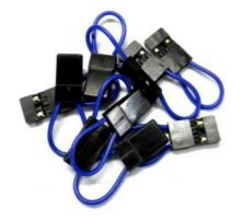
To select the throttle option, I've found these links on ebay, they're identical to Spektrum bind plugs: Please dont use standard 5.08mm header links as they short all 3 pins together!
