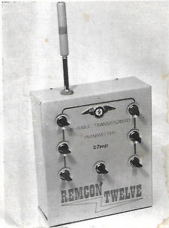
Remcon provide this clean looking case, dimpled for the keying switches to make "thumb twitching" more comfortable. The article gives dimensions for those who wish to do their own tin bashing.
