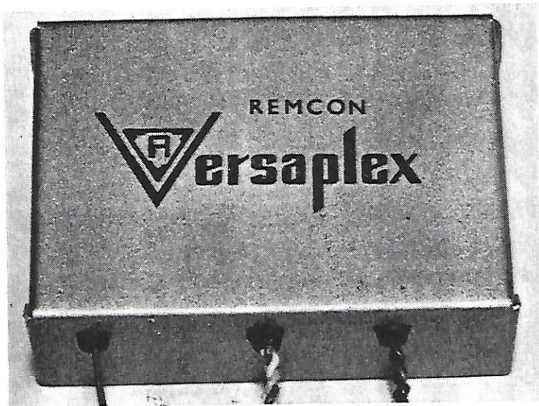
The completed receiver. Note substantial grommets to support wires.
